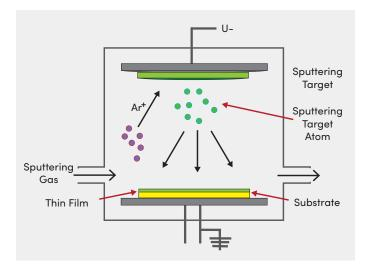
In the StenTech BluPrint™ PVD process, the wafer is exposed to one or more volatile precursors, which react and/or decompose on the substrate surface to produce the desired deposit.
